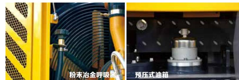
The ventilator is installed for the transmission, fuel tank, hydraulic oil tank, drive axle, and booster cylinder to make all systems clean and reliable.
