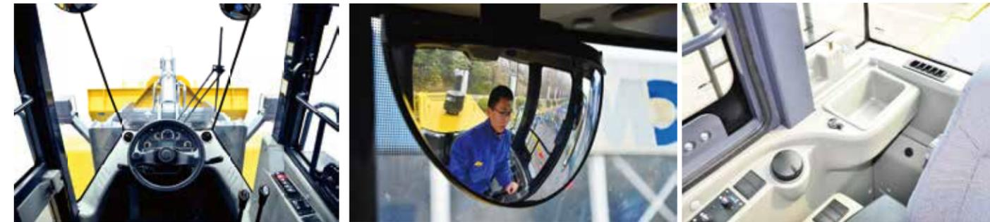
The full-coverage exquisite interior trim parts and the damping and noise reduction measures for the cab and engine hood reduce the noise by more than 6dB to meet the European cab internal noise standard and build a comfortable operating environment.
